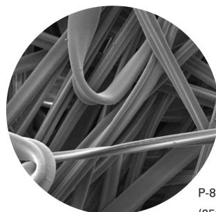
→ Needled 464 ml. Polyimide felt is a high temperature filtration media used in pulse jet baghouse dust collectors. This material performs well in dry, high heat applications. It is strong, abrasion resistant and good for applications up to 240°C.
