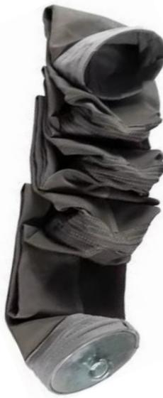
Fiberglass has moderate resistance to chemicals compared to other filter media materials. Although fiberglass filter bags have high tensile strength, they can't withstand flex abrasion from pulsing, which is remedied with a 20-wire cage.
