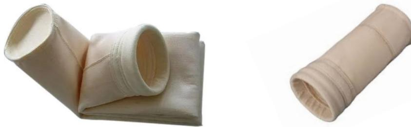
→ Used mainly in the temperature range 90 to 125°C in the presence of moisture/steam and mild acid conditions where polyester would fail due to hydrolysis. Homopolymer acrylic has a narrow window of application, typically drying, low temperature flue gas applications and some milling operations where moisture may be present.
