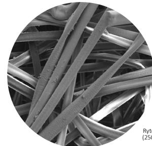
→ Needled 464 ml. PPS (polyphenylene sulfide) felt is a high temperature filtration media used in pulse jet baghouse dust collectors. This material performs well in applications where alkaline and/or chemical resistance is required. It also works well in applications with moisture content and where dew point crossings are common. It is strong, abrasion resistant with high resistance to alkalies and acids and good for applications up to 191°C.
