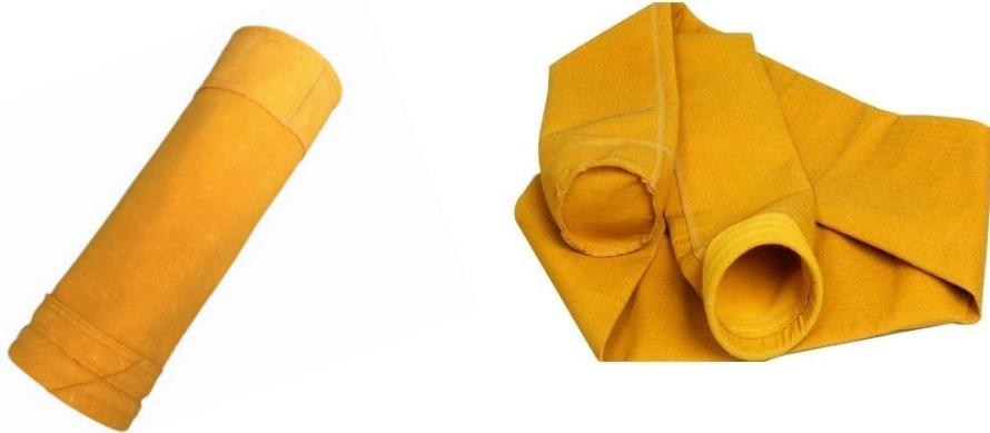
→ Needled 464 ml. Polyimide felt is a high temperature filtration media used in pulse jet baghouse dust collectors. This material performs well in dry, high heat applications. It is strong, abrasion resistant and good for applications up to 240°C.
